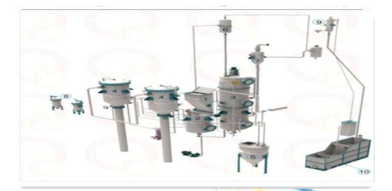
treatment called as degumming/neutralizing process. Thereafter the degummed oil is further processed in bleaching section under vacuum and treated with activated bleaching earth and carbon for reduction of color pigments. Next it will be deodorized under high vacuum. The edible oil obtained from Refinery
